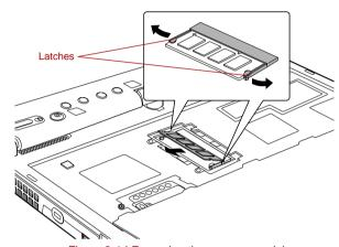
Figure 3-14 Removing the memory module
